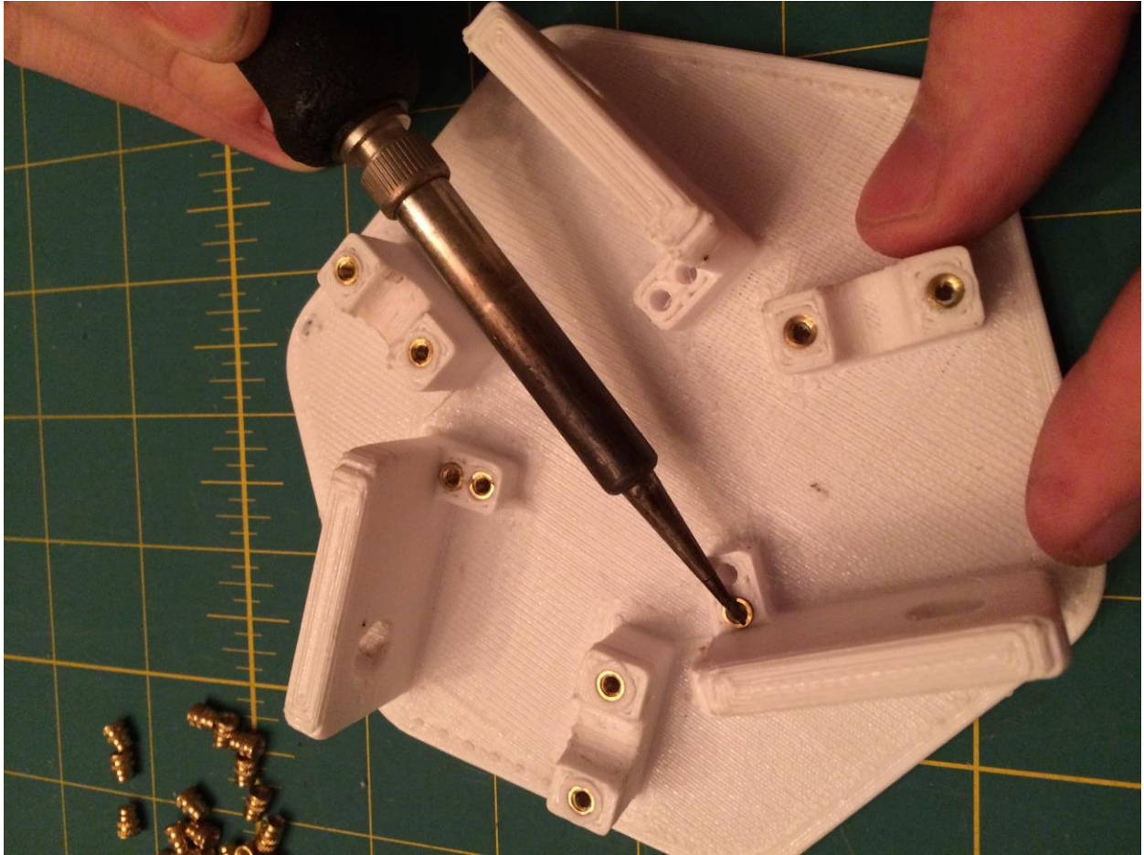
This particular insert requires holding the iron at a different angle
