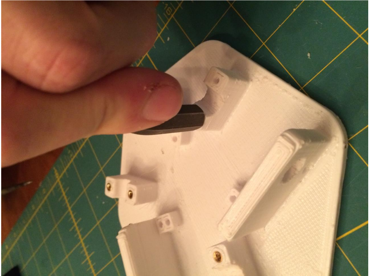
Using the top of a hex wrench to press the insert in flush with the plastic
